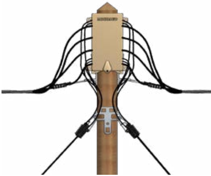
Network junction + service connections
