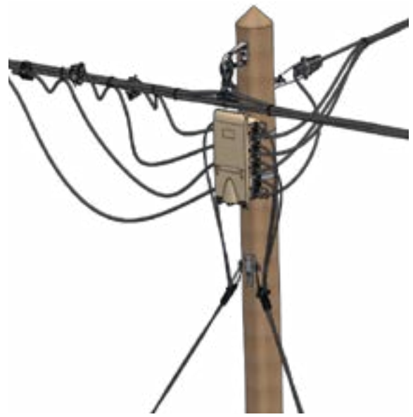
Network tapping + service connections
